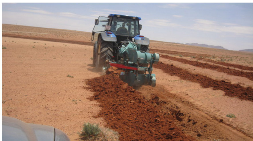
The Vallerani plow in action. The furrows capture rainfall and runoff water, encouraging range regeneration.
